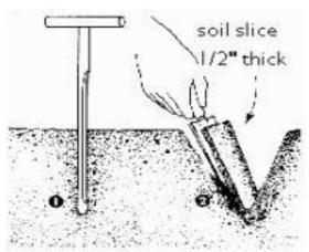
**(2) Shovel or spade:** Dig a V shaped hole to sample depth, and then cut a thin slice as shown below.
